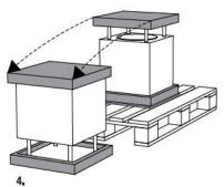
Holding the Cube2LV from the concrete body, NEVER from the base, gently turn the module, tilting it into upper position, WITHOUT removing the protective foam.
