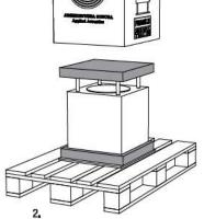
After removing the strapping securing the box to the pallet, lift and remove the box like in the image, leaving on the foam protecting the base.
