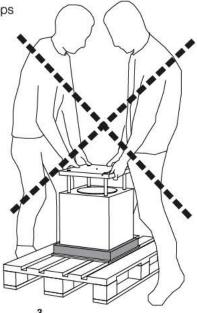
While turning the speaker, NEVER handle by its base, but only by its body! Do not remove the protective foam till the speaker is finally positioned.
