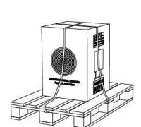
Due to its size and weight, the Cube2LV Sub is shipped in a box secured to a pallet with strapping to allow its handling and movement into position with a forklift.
